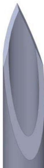
Figure 1-3. Standard three-planed bevel hypodermic needle tip geometry.
